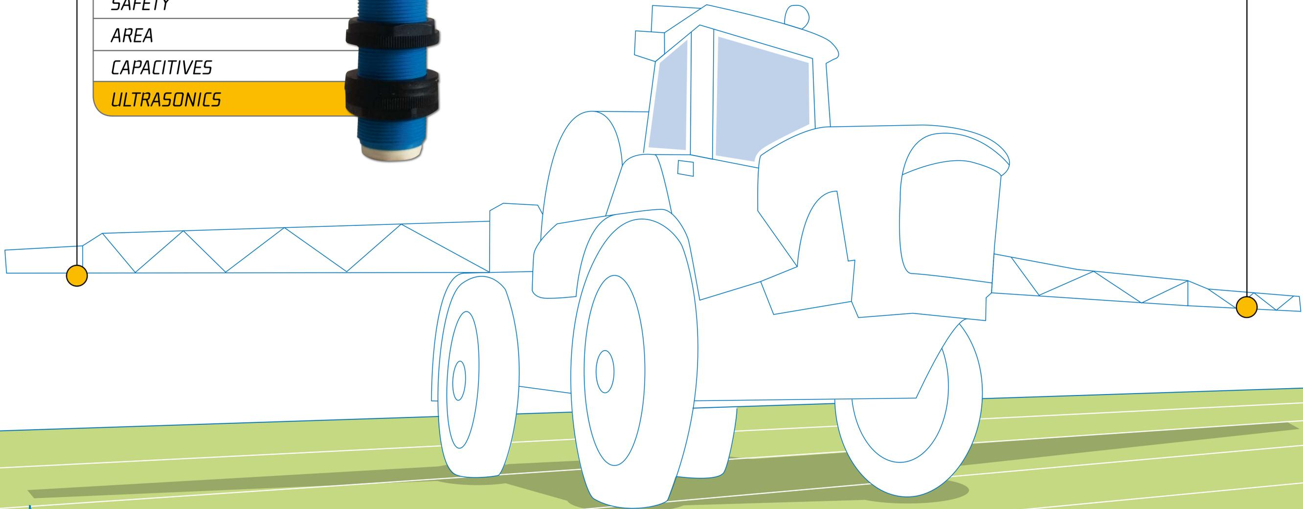
In the agricultural machine for spread of herbicidal TU1 ultrasonic sensor **is the best application to notice the presence and the height of the plantations**. TU1 is placed at the extremities of machine and it can automatically puts the diffuser in a safety position both effecting U-turn and when working on uneven road surface. You can thus reduce risks and costs.
