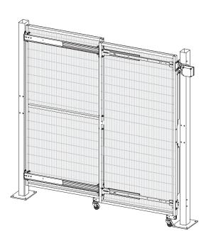
Door that combines the rotation and sliding of door leaves in a single movement. Ideal for layouts where the space to perform these movements is limited.
