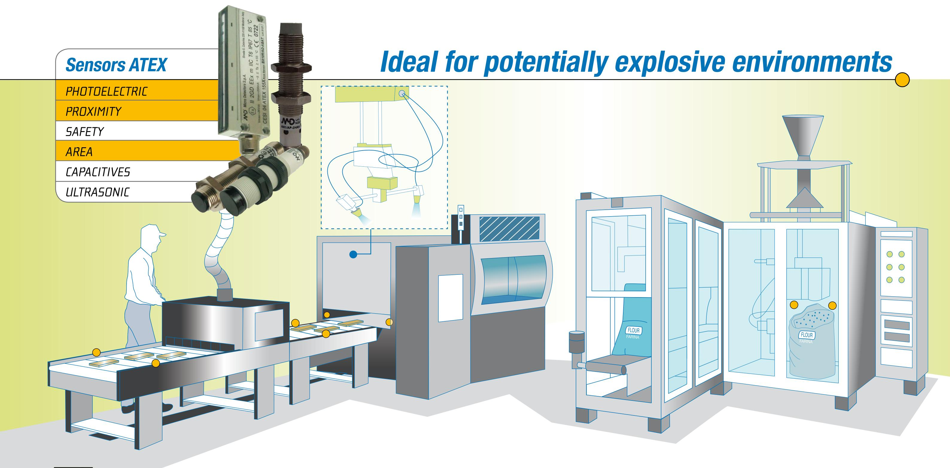
Inductive, photoelectric and area sensors with ATEX Category 3 certification could be used in presence of explosive atmospheres caused by gas and powder. Which are their applications?
