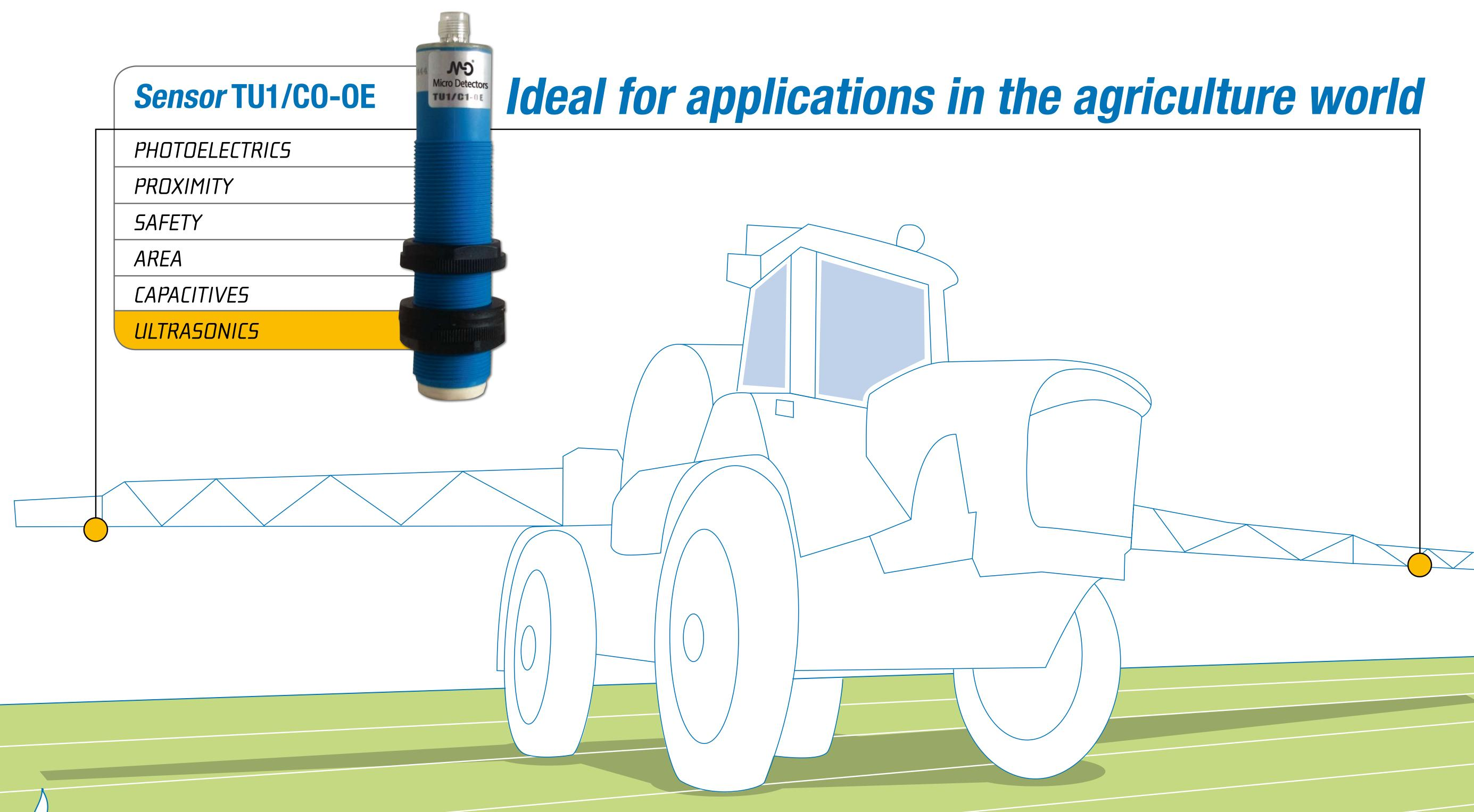
In the agricultural machine for spread of herbicidal TU1 ultrasonic sensor is the best application to notice the presence and the height of the plantations. TU1 is placed at the extremities of machine and it can automatically puts the diffuser in a safety position both effecting U-turn and when working on uneven road surface. You can thus reduce risks and costs. MD. Sensors serving industrial automation.
